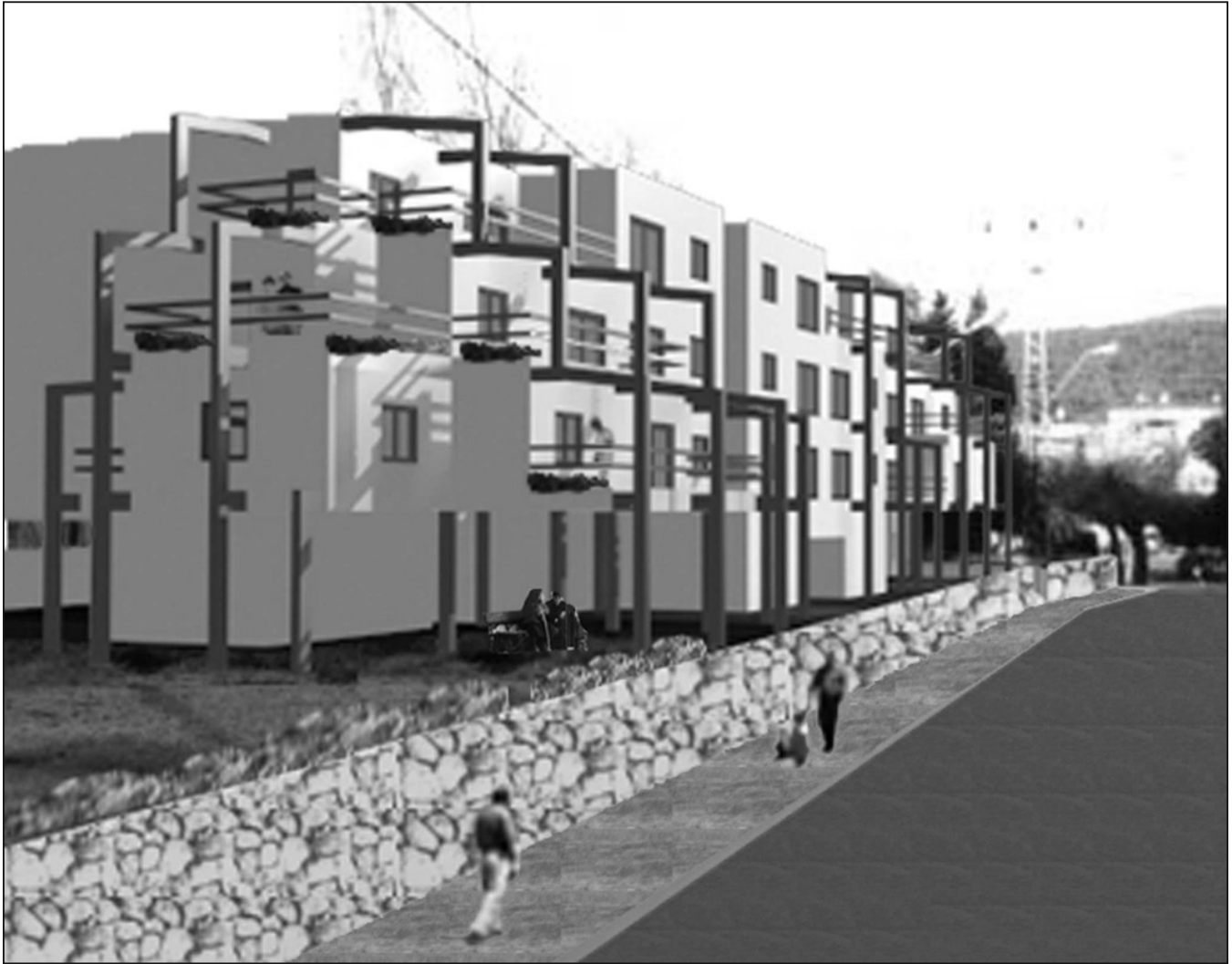
FIGURE 6. A computer simulation of preprovision of supports for independent enlargements in a multiunit building in the moderate-income small town of Migdal HaEmek. (Courtesy of architects Avi Sela and Eyal Nir.)
